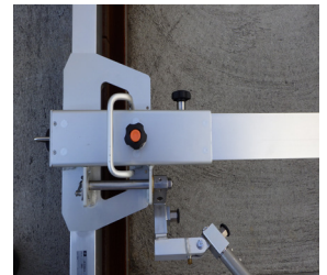
Easy to assemble, simply install Gauge beam and Push-rod to Measurement beam.
