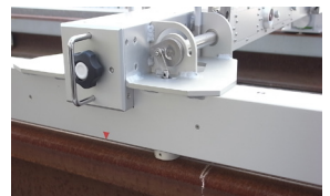
Brake shoe contacts the rail when Rush-rod falls down.
